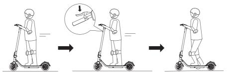
Lightly press the throttle lever on the right hand side to speed up, remember not to be too fast. Pinch the brake lever to brake. (Be careful not to brake suddenly when riding.) When the scooter stops or slows down, put down one foot and get off the scooter normally.
