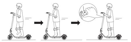
Stand on the deck with one foot, push the other foot back on the ground and start sliding. The motor can only start after the vehicle speed reaches 3km/h (1.86mph). Lightly press the throttle lever on the right hand side, the scooter will accelerate (harder you push ~ greater the speed), and the steering can control the riding direction (similar to a bicycle).
